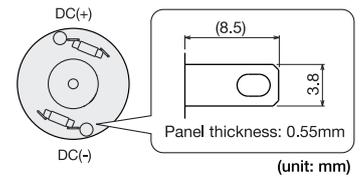
Caution: Short circuit between terminals may occur due to end of motor life or short circuit between commutator slits by specific operating environment and condition. In order to prevent circuit burnout, please take protective measures such as using fuses.
